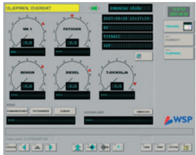
Wonderware InTouch HMI visualizes the discharge process and the pressure monitoring
