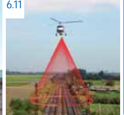
6.11 Laserscanning of Highway 45, Trollhattan Airborne laserscanning to generate terrain modelling.
