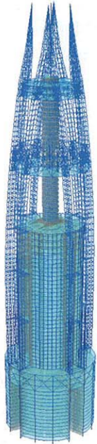
Finite Element Analysis Model of Spire and Crown.
